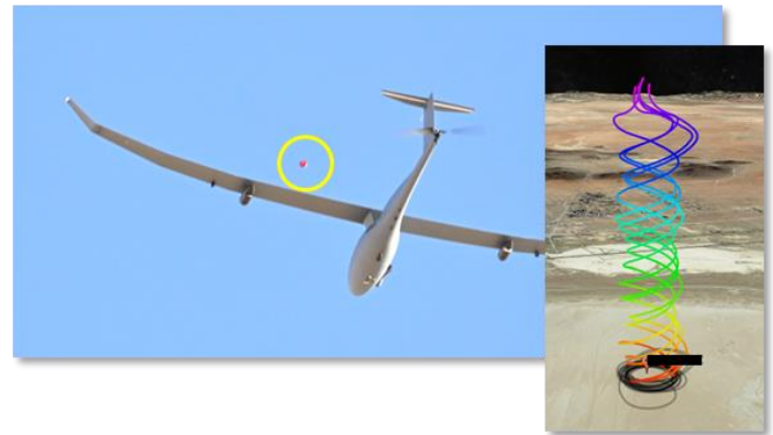
Vanilla deploying air-dropped micro-UAS; Micro-UAS glide paths controlled via BLOS Vanilla node
