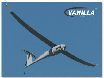
Vanilla Unmanned holds official and unofficial world records for endurance, and is capable of flights up to 10 days covering 15,000 nm. The multi-mission heavy-lift variant which completed this 73.5 hr flight can carry payloads across multiple internal and external mounts, enabling multi-day, multi-INT missions on a single flight.
